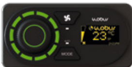
Ventilation function active panel
